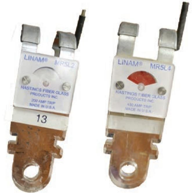
After a blink, if the indicator on a fault-finder remains white, left, it indicates to the technician that the fault is farther up the line. If the indicator turns red, right, the technician knows he has narrowed the fault to a smaller area and adjusts his search accordingly. The process is repeated until the fault is located and repaired.
